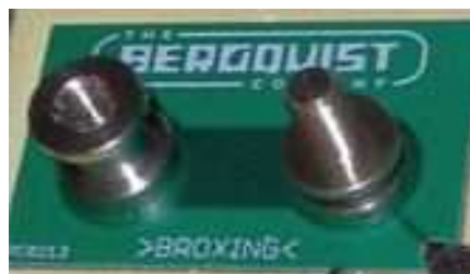
perfect contact-surface after soldering with BroxAlloy galvanization
