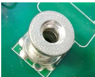
melted contact surface at tinned contact
